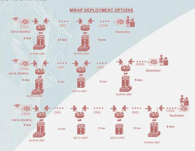
The antenna system is a flat panel and is both Horizontal or Vertical polarized. The 5 GHz band is for back haul operation only.
