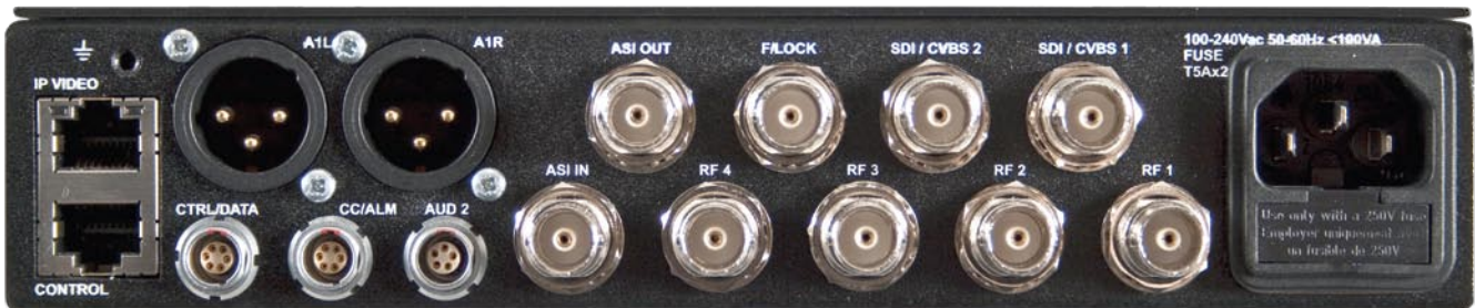
HDR-4000 Diversity Receiver Connections
